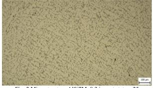
Fig. 2 Microstructure AlSi7Mg0.3 in cast state - 25
