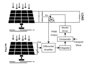
Fig. 4. PV pilot concept
