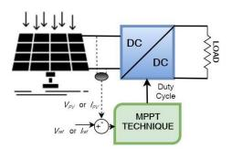
Fig. 7. Voltage/current feedback method
