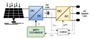
Fig. 13. DC-link capacitor drops control method diagram
