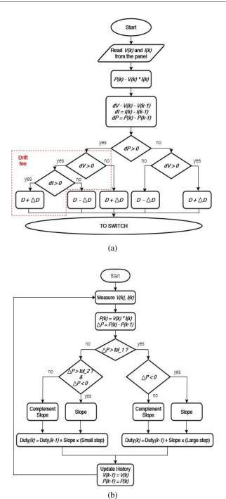
Fig. 12. Flowchart systems are proposed by: (a) literature [29] to eliminate drift and (b) by [67] to reduce oscillations
