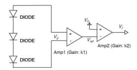
Fig. 9. Control circuit configuration based on constant voltag
