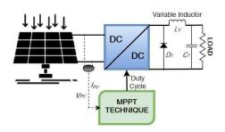
Fig. 14. Variable inductance method diagram
