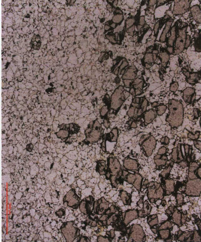
Microscopic photograph of light granulite and garnetite
