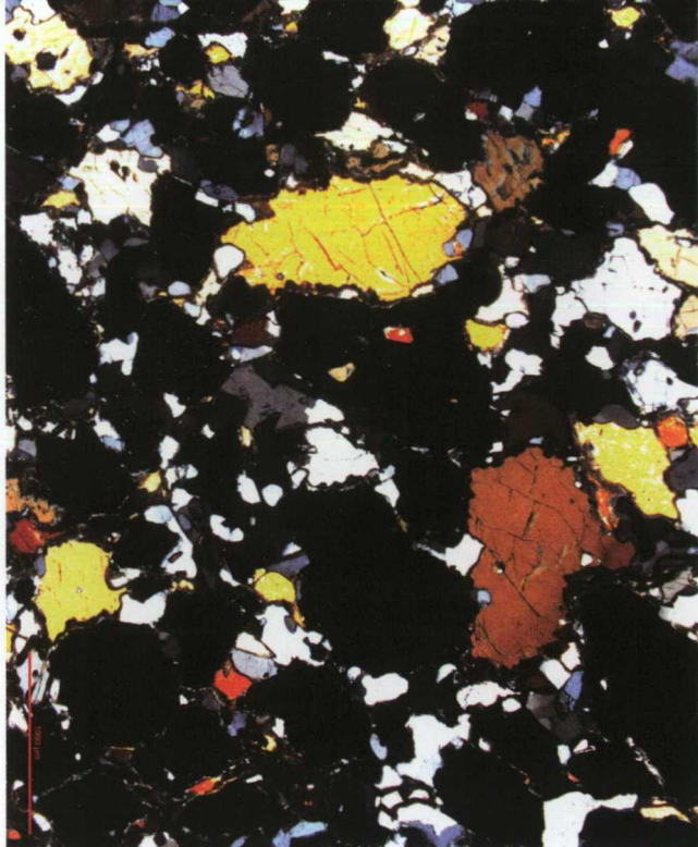
Microscopic photograph of eclogite
