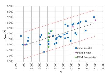
Fig. 6. Experimental results; force  $F_{\text{max}}$  as a function of sample stiffness S; the pink (magenta) color marks the results of numerical calculations estimating the values  $E_{\text{bit}}^S = E_{\text{bit}}^S(S)$ ; the results that estimate the values  $F_{\text{max}}^S = F_{\text{max}}^S(S)$  are marked green
