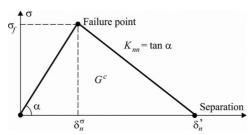
Fig. 7. Cohesive contact linear damage evolution model [Abagus]
