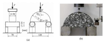
Fig. 1. The scheme of semi-circular bending test (a) and view of the test sample (b)
