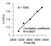
Fig. 8. Numerical adjustment of  $\sigma_f^S$  values, taking into account the dispersions around the mean values: five F - d plots and the corresponding values  $\sigma_f^S$ , linear relationship  $\sigma_f^S - F_{\text{max}}$
