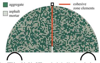
Fig. 5. Two-phase FEM model of the SCB sample obtained by the randomly generated elements
