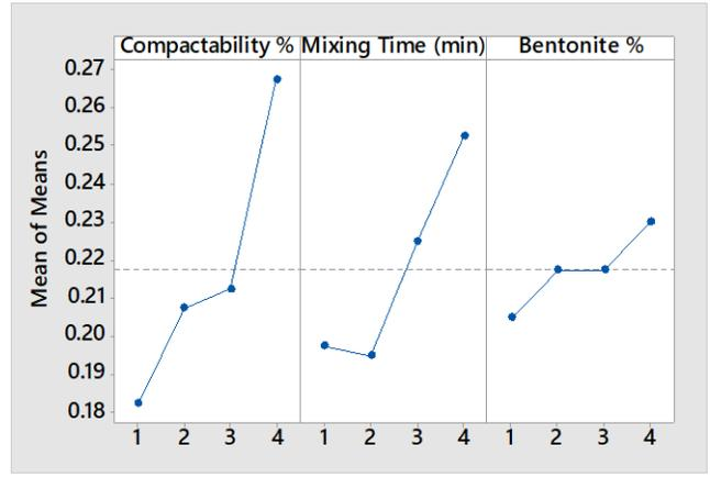
Fig. 6. Main effect of parameters on Tensile strength
