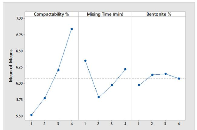
Fig. 2. Main effect of parameters on Permeability
