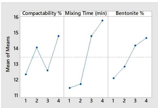
Fig. 4. Main effect of parameters on compressive strength
