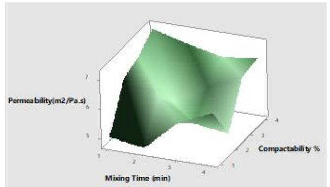
Fig. 1. Permeability Vs compactability &amp; Mixing time
