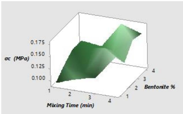
Fig. 3. Compressive strength Vs Bentonite &amp; Mixing time
