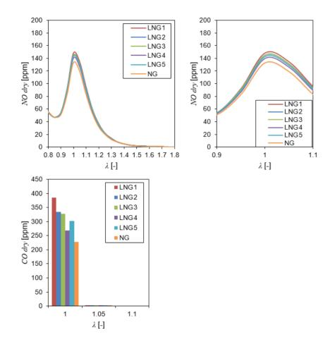
Figure 3: Emission characteristic of NO and CO; 1D FreeFlame with the radiative heat loss.
