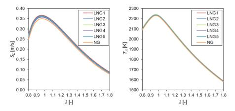
Figure 1: Laminar flame speed and adiabatic flame temperature versus air excess ratio.
