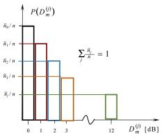
Fig. 6. Histogram of modulation depths. The probability  $P = \hat{n}_0/n$ , obtained for  $D_m = 0$ , corresponds to nonmodulated intervals  $\tau$  (Fig. 3).
