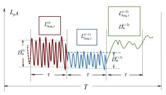
Fig. 3. Time variation of A-weighted sound level  $L_{pA}$  characterized by series of pairs,  $L_{Aeq.\tau}^{(i)}$ ,  $D_m^{(i)}$ .
