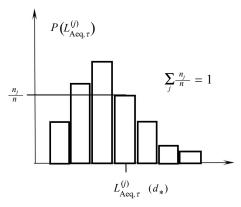
Fig. 5. Histogram of short-term A-weighted time-average sound levels at the reference distance  $d_*$ .
