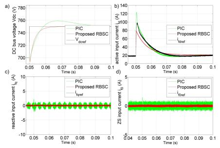
Fig. 6. Comparison of DC bus voltage and input currents performance under DC-bus voltage reference change from 700 V to 750 V at 0.05s when the DC capacitor is 3  $\mu$ F.
