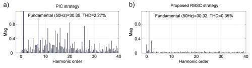
Fig. 10. Grid currents THDs under  $C_{dc} = 6 \ \mu\text{F}$  when the load is changed from 100 to 50  $\Omega$ . a) PIC strategy, b) the proposed RBSC strategy.
