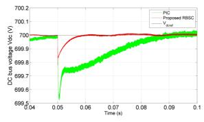
Fig. 9. Comparison of FLVSR DC bus voltage performance with the traditional PIC strategy and the proposed RBSC strategy under load change from 100 to 50  $\Omega$  with  $C_{dc}$  = 6  $\mu$ F.
