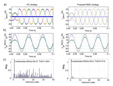
Fig. 8. Grid currents, first-phase grid voltage and its corresponding current, and the harmonic spectrum of grid currents under load change from 100 to 50  $\Omega$  at 0.05 s. PIC strategy (on left), proposed RBSC strategy (on right).
