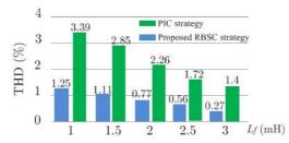
Fig. 11. Comparison of grid currents THDs versus filter inductor variation with the PIC and the proposed RBSC.
