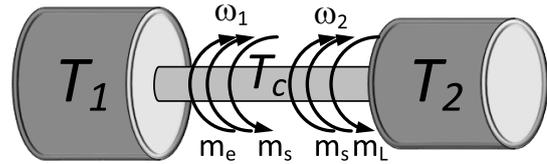
Fig. 1. Schematic diagram of two-mass mechanical system
