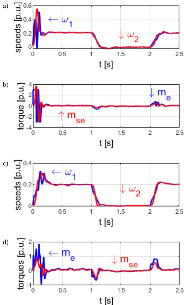
**Fig. 8.** Transients from the adaptive control system: the motor  $\omega_1$  and load  $\omega_2$  speeds a), c) driving  $m_e$ , and shaft torque  $m_s$  in the system working with single EKF a)–b) and working with fuzzy MKF c)–d)
