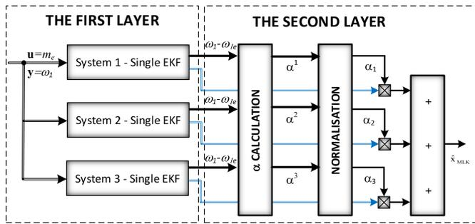
Fig. 3. Block diagram of MKF
