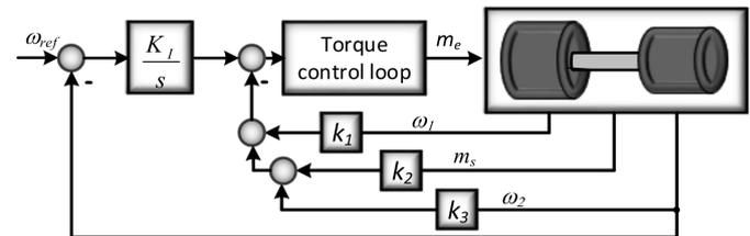
Fig. 2. Block diagram of the considered control system
