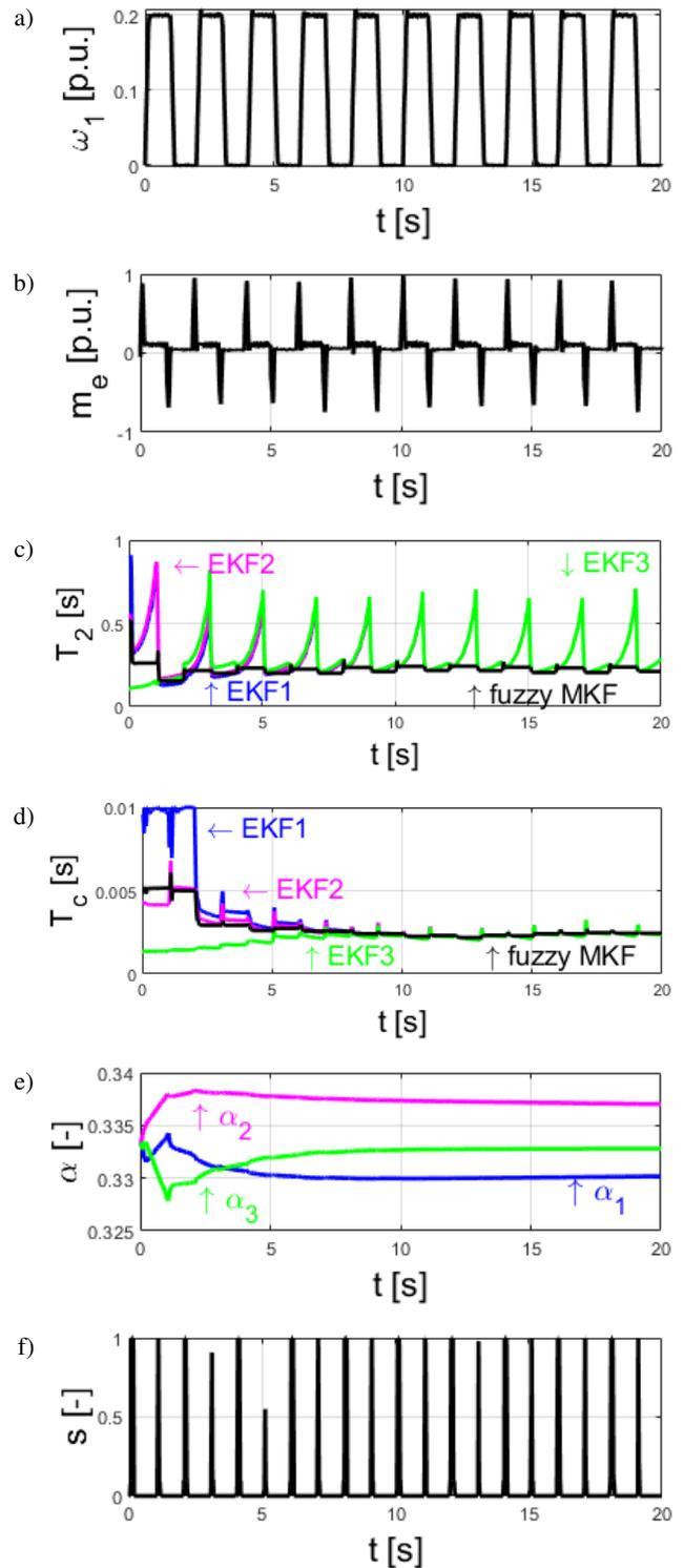
**Fig. 7.** Experimental results: a), b) – the transients of the driving motor speed  $\omega_1$  and electromagnetic torque  $m_e$ , c), d), – the transients of the  $T_2$ ,  $T_c$  parameters identification with close-ups, e) – the transients of weight coefficients, f) – the transient of the state recognition system output signal
