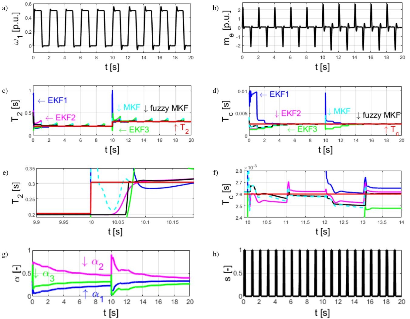
**Fig. 5.** Transients of the motor speed  $\omega_1$  (a); and driving torque  $m_e$  (b); estimated values of the time constant of load machine  $T_2$  (c),(e); elasticity time constant  $T_c$  (d),(f); weight coefficients (g), and output detection system (h)
