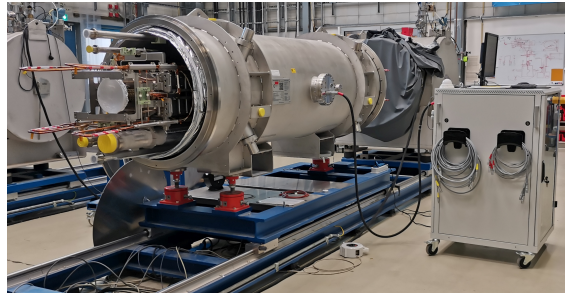
Fig. 1. Superconducting SIS100 dipole magnet at the test bench in GSI Darmstadt, Germany
