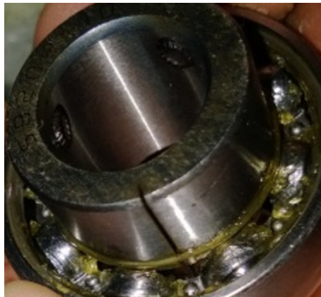
Fig. 3. 0.5 mm fault at inner race
