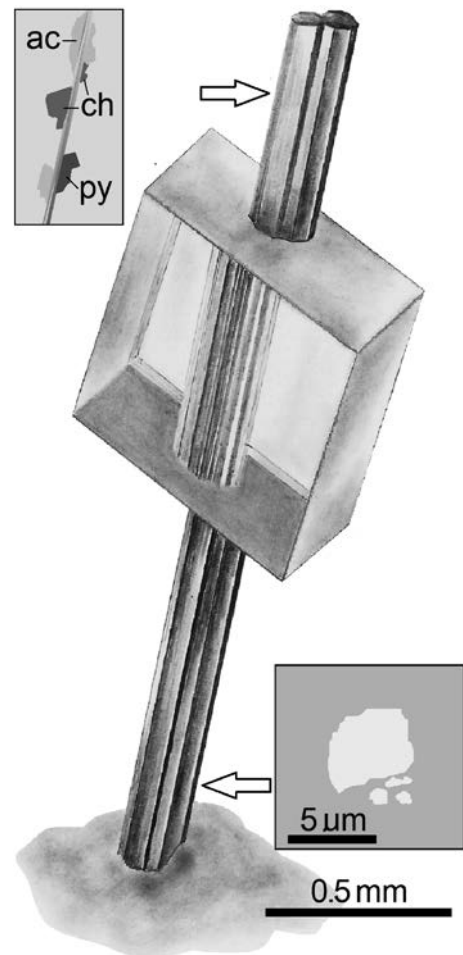
Text-fig. 16. Adhesion of two parallel native silver rods partly overgrown by calcite crystal of rhombohedral habit; note the high birefringence effect visible in the calcite crystal. The BSE image inserts show inclusions of Ag-including gold (electrum), found in the lowest part of the silver rods, and acanthite (ac), chalcopyrite (ch) and pyrite (py) inclusions formed along the contact zone (straight strip) of the upper parts of the rods; Rybień Mt.
