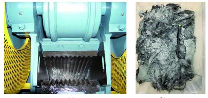
(a) (b) Fig. 4. Jaw crusher (a) and material after crushing process (b)
