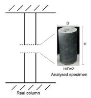
Fig. 2. Cylindrical specimen as a fragment of column
