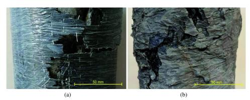
Fig. 7. The course of destruction of samples strengthened by CFRP (a) and carbon fibre scraps (b)
