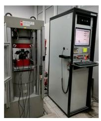
Fig. 6. Testing machine used in compression tests
