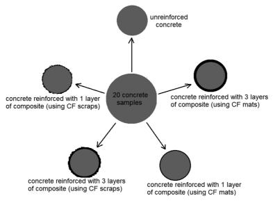
Fig. 3. Type of analysed group of specimens
