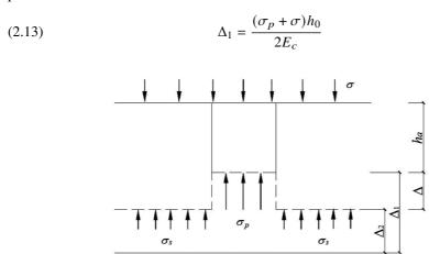
Fig. 3. The force diagram of cushion layer
