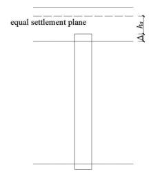
Fig. 1. Deformation diagram of composite foundation
