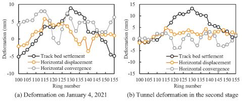
Fig. 10. Variation of the tunnel deformation caused by the second stage grouting
