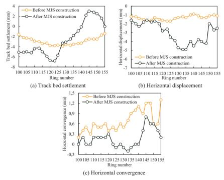
Fig. 8. Comparison results of damaged TBM tunnel deformation
