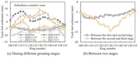
Fig. 13. Track bed settlement under different grouting stages
