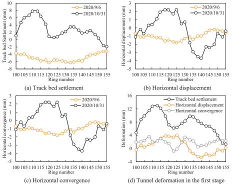
displacement and convergence are relatively small, and no more than 4 mm in the first stage.
