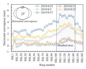
Fig. 5. Horizontal convergence ( $\Delta D$ ) of the affected up-track TBM tunnels
