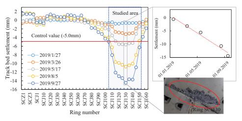
Fig. 3. Track bed settlement of the affected up-track TBM tunnel
