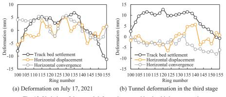
Fig. 12. Variation of the tunnel deformation caused by the third stage grouting
