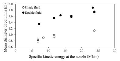
Fig. 4. Mean diameter of columns versus specific kinetic at the nozzle
