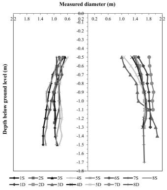
Fig. 3. Columns diameters profiles of single (left) and double fluid (right) columns versus depth
