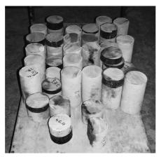
Fig. 8. Cylindrical samples of jet grouted material prepared for uniaxial compressive tests [19]
