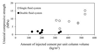
Fig. 9. Uniaxial compressive strength as function of the cement injected in the unit volume of column
