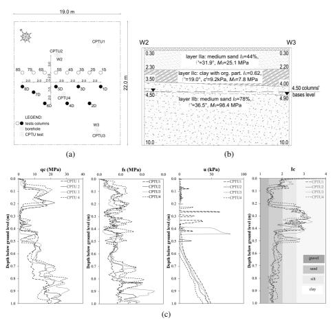
Fig. 1. (a) plan view of the Bojszowy Nowe test site with the layout with jet grouting columns, boreholes and CPTU tests, (b) geotechnical scheme of the subsoil, (c) CPTU profiles and interpretation with Robertson [23]
