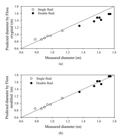
Fig. 5. Comparison between measured and predicted diameter for single (SF), double fluid (DF) jet grouting columns. Prediction has been performed with Eq. (2.2) and Eq. (2.3) assigning the parameters of Table 2 (a) and modifying the exponent  $\beta$  to 0.24 (b)
