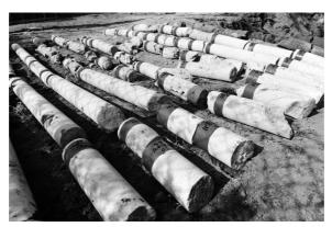
Fig. 6. Core samples of jet grouted material from trial field in Bojszowy Nowe [19]
