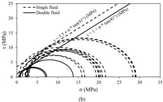
Fig. 7. High pressure triaxial device and sample of jet grouting material equipped with extensometers [19] (a), failure envelope for single and double fluid jet grouting (b)
