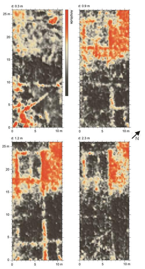
Fig. 6. Selected time slices (GPR plans) for 0.3–2.3 m depth (processing and interpretation by F. Welc).
