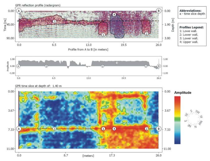
Fig. 8. GPR plan (time slice) prepared for a depth of approx. 1.4 m compiled with reflection profile no. 29, records of the relative amplitude value and interpretation (drawing and interpretation by F. Welc).
