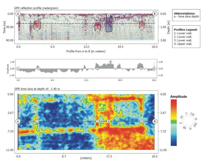
Fig. 7. Time slice prepared for a depth of about 1.4 m, juxtaposed with reflection profile no. 22, with records of the relative amplitude value and interpretation (drawing and interpretation by F. Welc).
