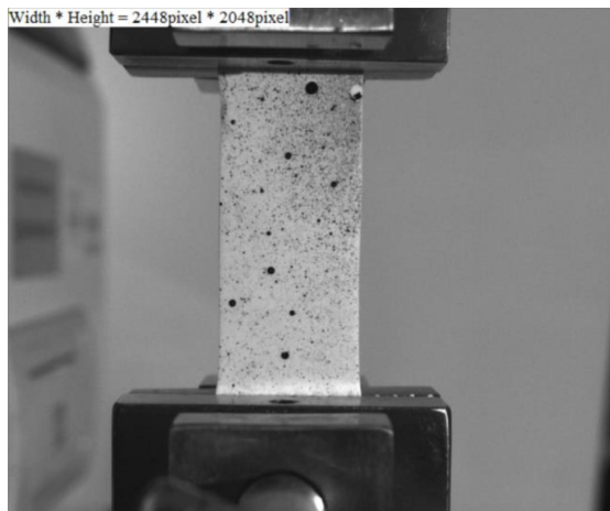
Fig. 7. DIC tensile test of ZnS:Cu 2+ -PDMS mechanoluminescent film.
