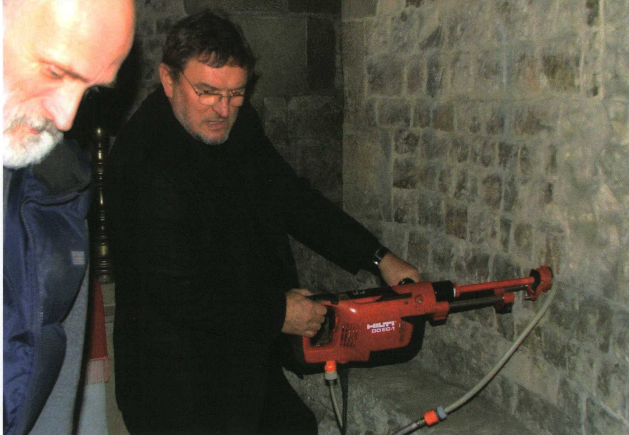
Collecting original mortar samples from deep inside a rebuilt wall. Research team members Wiesław Procyk and Andrzej Koss (right)
