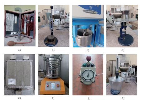
Fig. 1. Tovarov device (a), Vicat apparatus (b), mixer (c), flow table (d),  $40 \times 40 \times 160$  mm prism filled in with reference mortar (e), standard sieves (f), air content meter (g) and standard cone apparatus (h) were used to determine the properties of mortar and its constituents
