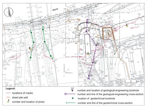
Fig. 2. Map of the distribution of deformations in the subsoil of the Warta side in Wronki [12]
