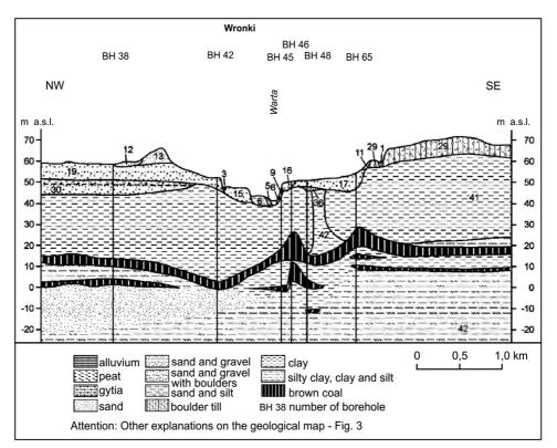
Fig. 5. The fragment of the C–D geological cross-section [6]
