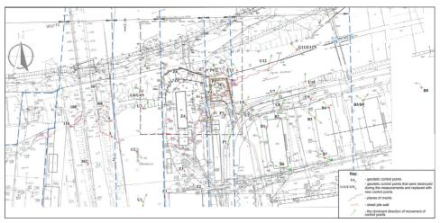
Fig. 7. Distribution of geodetic control points [13–15]
