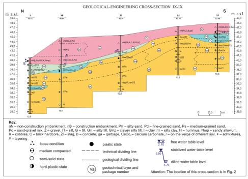
Fig. 6. The fragment of the geological engineering cross section IX-IX (modified) [16]
