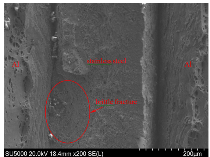
Fig. 8. The tensile fracture morphology of the multilayer composites obtained by explosive welding with explosive of 20 mm thickness
