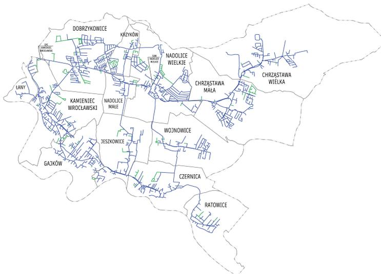
Fig. 4. Water-pipe network structure in the Czernica community
