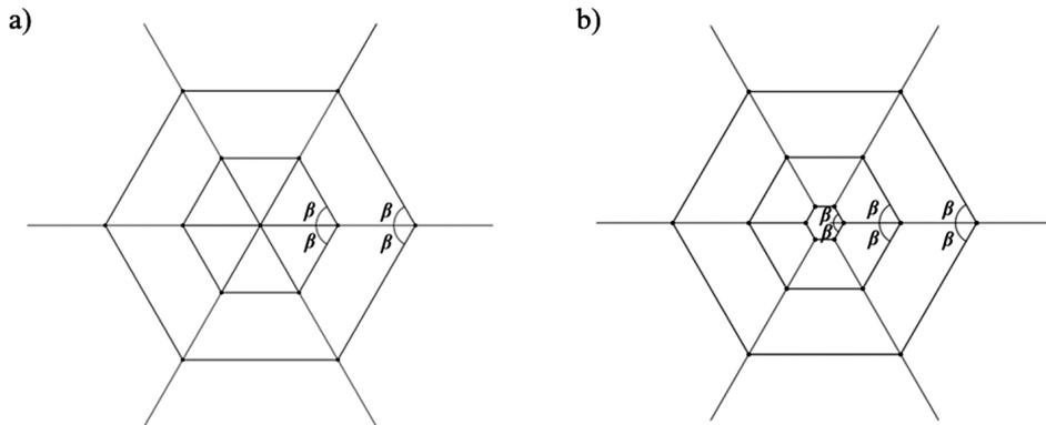
Fig. 4. View from the top of the regular Geiger domes: a) RG 6A, b) RG 6B
