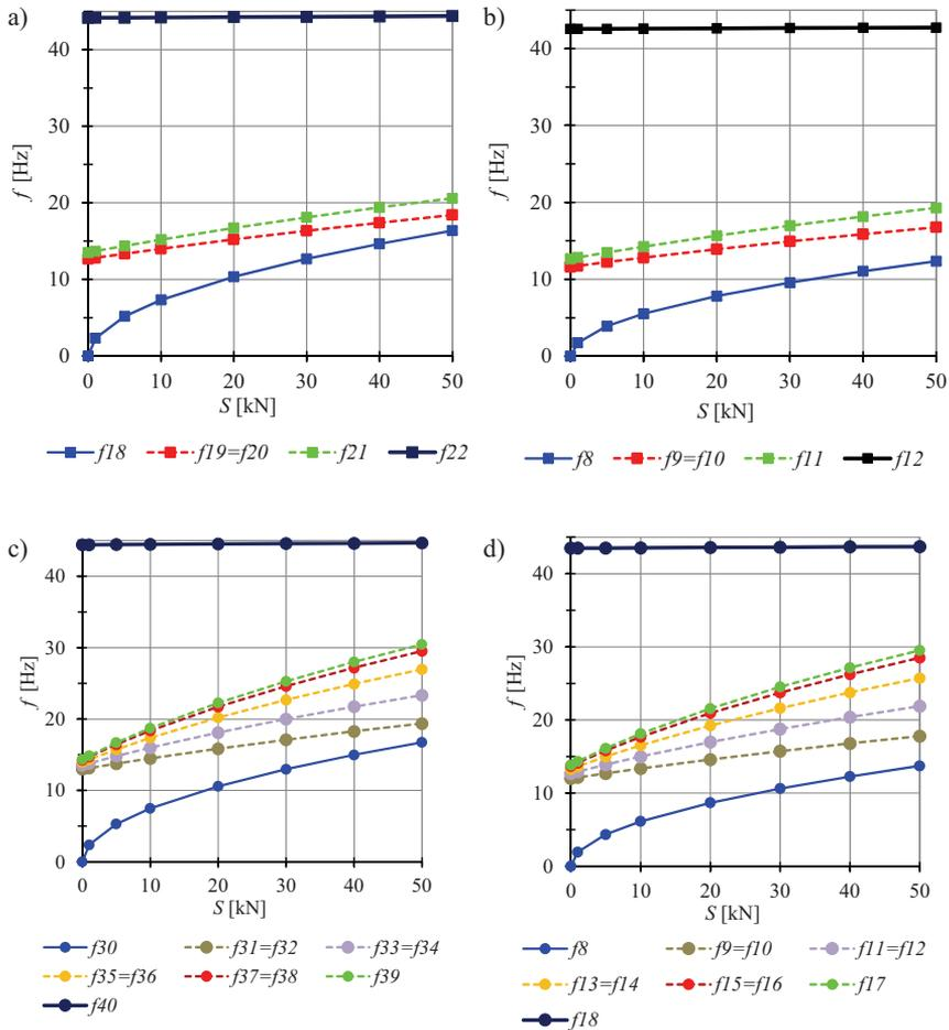
Fig. 7. Influence of the initial prestress  $S$  on the natural frequency: a) RG-6A, b) MG-6A, c) RG-12A, d) MG-12A
