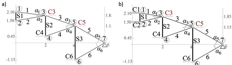
Fig. 1. Load-bearing girders of Geiger dome: a) type A, b) type B
