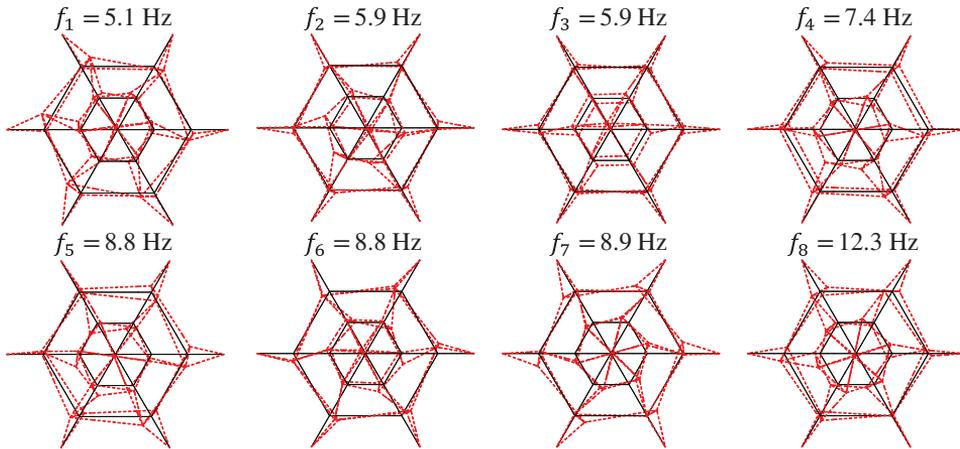
Fig. 6. Forms of vibration for the MG 6A dome (values of frequencies for  $S_{\max}$ )
