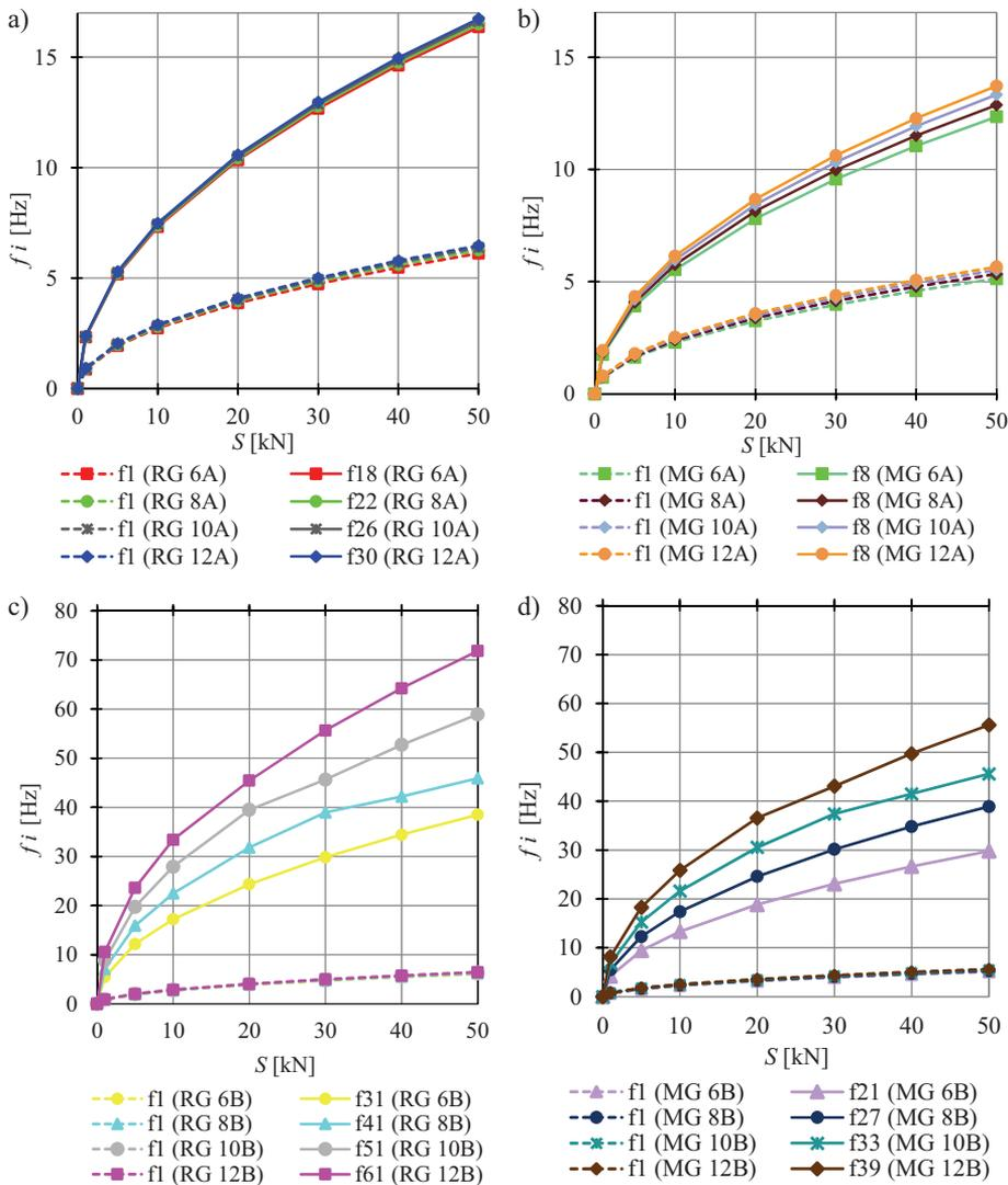
Fig. 5. Influence of the initial prestress  $S$  on the natural frequency: a) RG iA, b) MG iA, c) RG iB, d) MG iB
