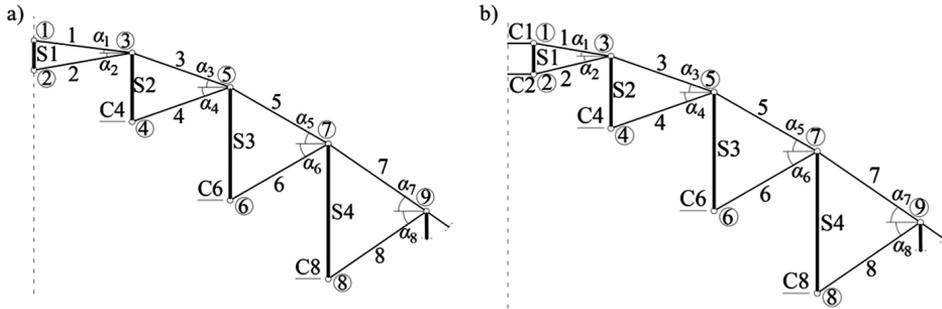
Fig. 3. Load-bearing girders of the Geiger dome: a) type A, b) type B
