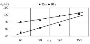
Fig. 2. Development of green compressive strength depending on mixing time
