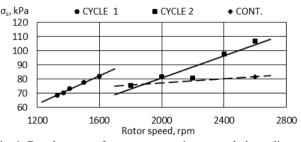
Fig. 1. Development of green compressive strength depending on the rotor speed
