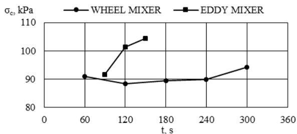
Fig. 5. Development of green compressive strength
