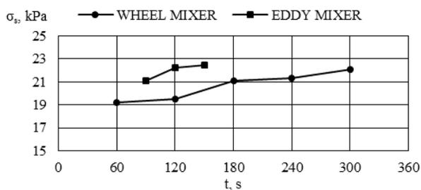
Fig. 7. Development of green Shear strength
