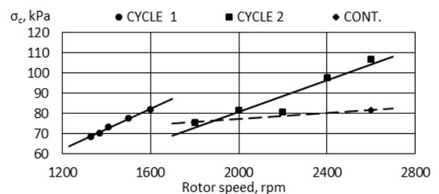
Fig. 1. Development of green compressive strength depending on the rotor speed
