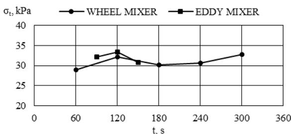
Fig. 6. Development of green split tensile strength
