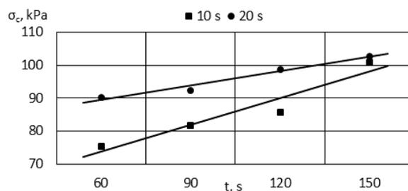
Fig. 2. Development of green compressive strength depending on mixing time
