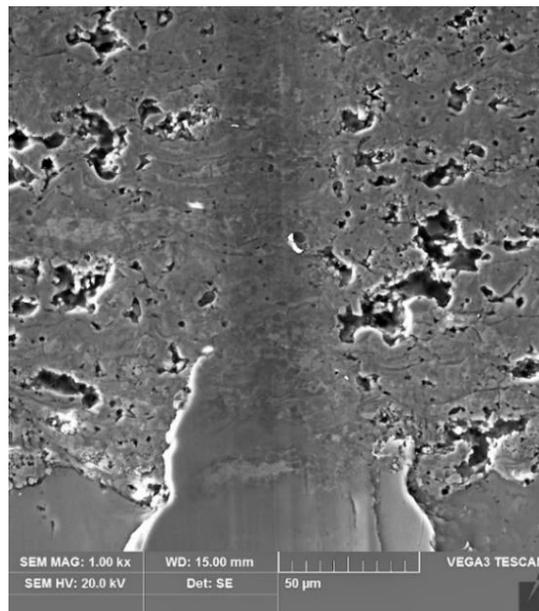
Fig. 9. View of the scratch in the area of the substrate-coating transition boundary
