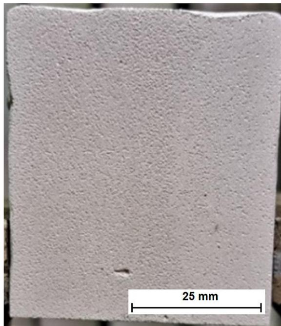
Fig. 5. View of the surface of the  $\text{Al}_2\text{O}_3\text{-TiO}_2$  coating applied to the  $\text{AlSi7Mg}$  alloy casting
