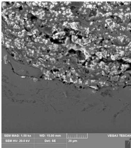
Fig. 6. SEM image of the Al<sub>2</sub>O<sub>3</sub>-TiO<sub>2</sub> coating applied to a casting made of the AlSi7Mg alloy
