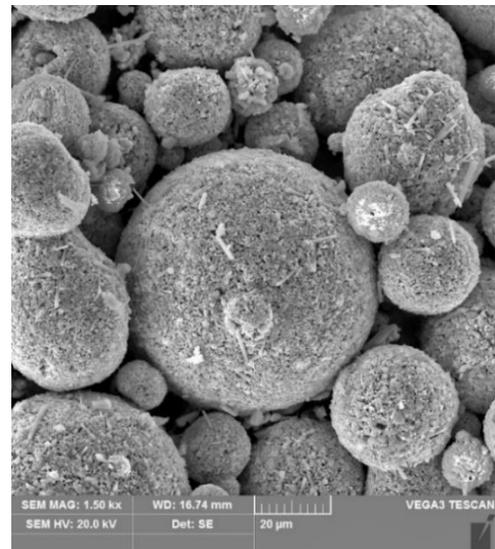
Fig. 3. SEM image of the Al<sub>2</sub>O<sub>3</sub>-TiO<sub>2</sub> powder
