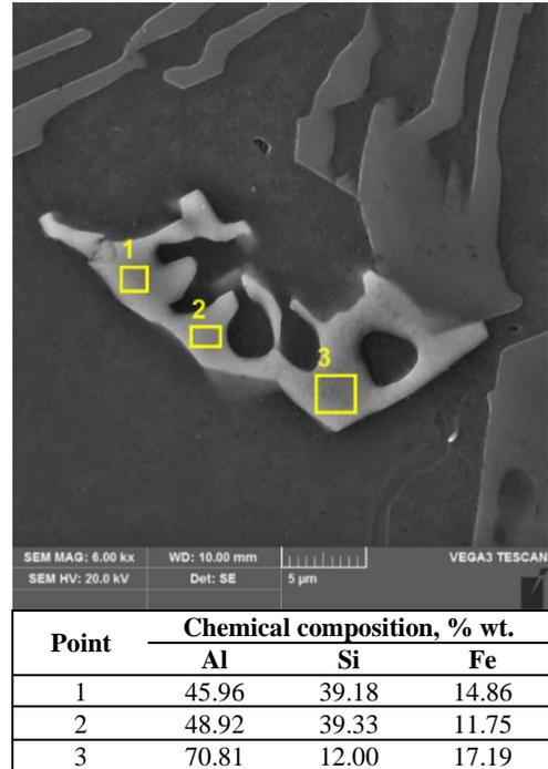
Fig. 2. Results of the X-ray microanalysis of intermetallic phases in the microstructure of the AlSi7Mg alloy
