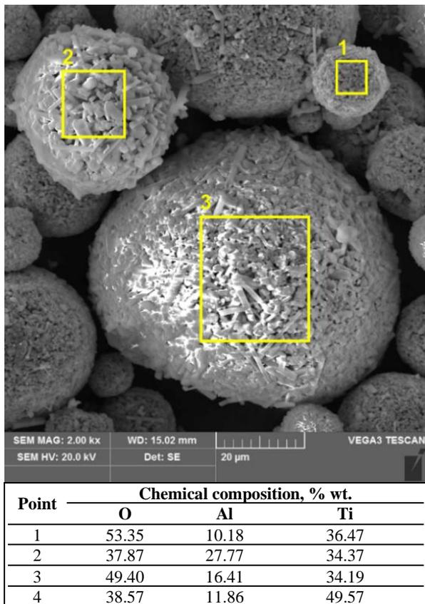
Fig. 4. Results of the X-ray microanalysis of the  $\text{Al}_2\text{O}_3\text{-TiO}_2$  powder
