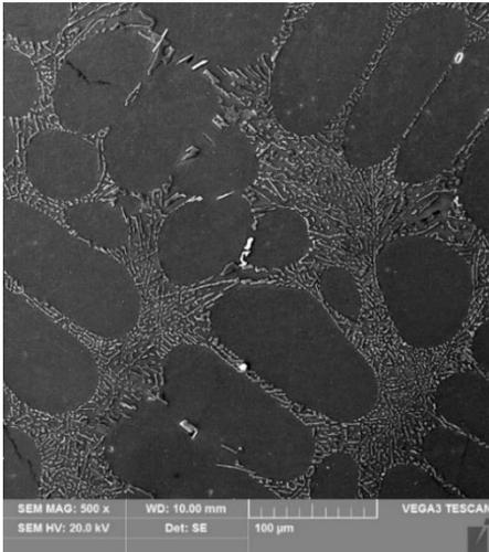
Fig. 1. SEM image of an example microstructure of the AlSi7Mg alloy
