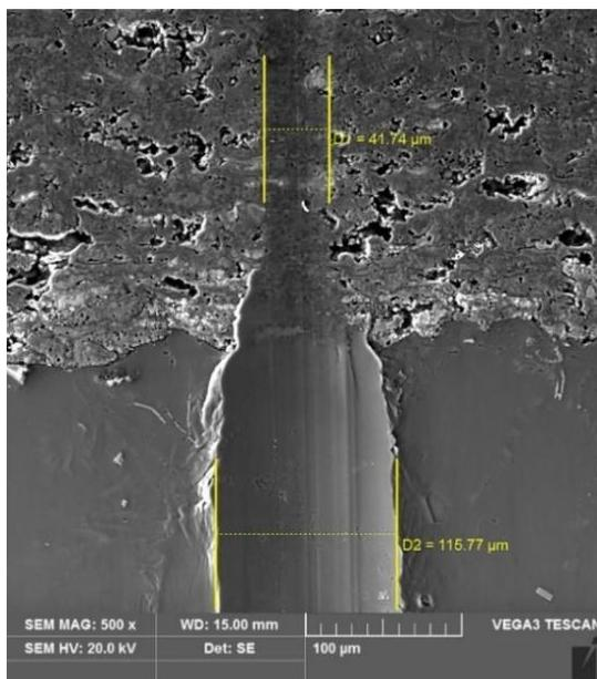
Fig. 10. Results of measurements of the scratch width in the substrate and the coating
