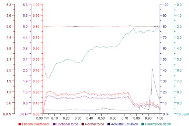
Fig. 8. Changes in scratch test parameters during scratching of the substrate material and coating
