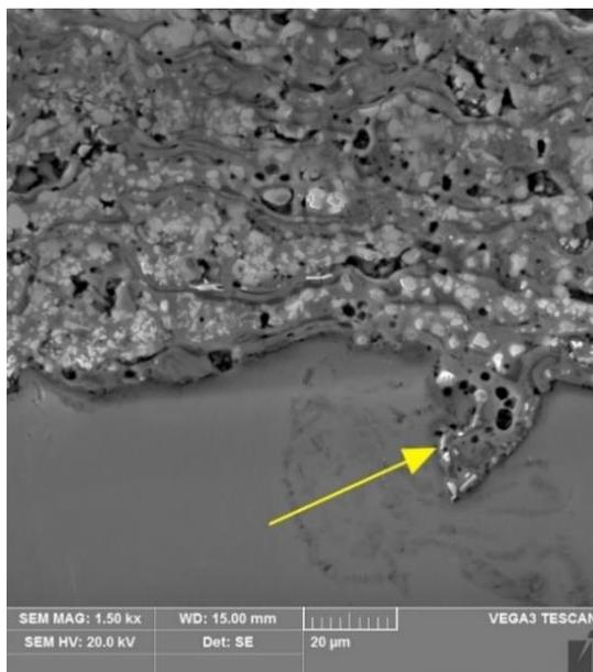
Fig. 11. View of the Al<sub>2</sub>O<sub>3</sub>-TiO<sub>2</sub> coating with characteristic hooks indicated by an arrow in the figure
