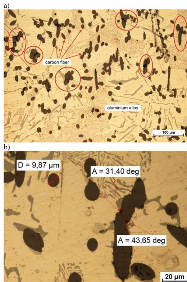
Fig. 8. Micrographs of the Al/CF composite with marked areas of porosity - a), wedge-shaped metal-free capillaries - b)
