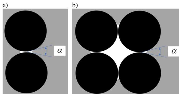
Fig. 9. Two fibers forming a capillary that is difficult to wet – a), fibers blocking the flow of metal - b)
