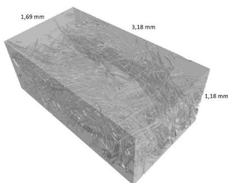
Fig. 7. Microtomography of a sample cut from an Al/CF cast with visible areas of structure discontinuity (dark area)
