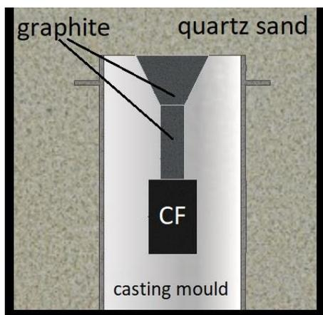
Fig. 4. Scheme of mold protection during the firing process
