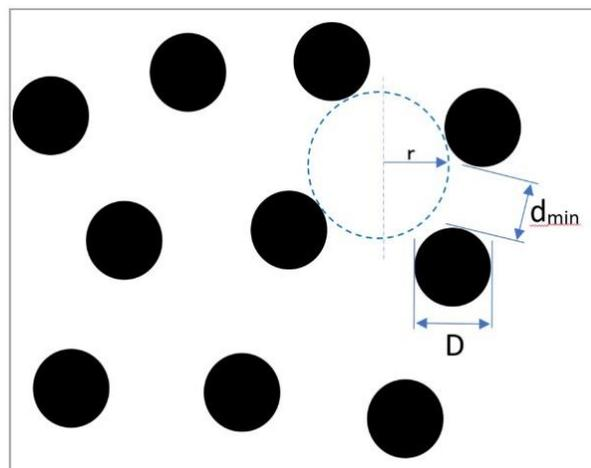
Fig. 1. An example layout for a space limited by reinforcement fibers (of diameter  $D$ ), where  $d_{min}$  is the smallest distance between them
