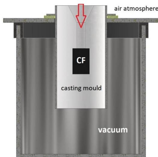
Fig. 6. Scheme of the vacuum casting station: the red arrow indicates the direction of pouring and the atmospheric pressure acting on the metal
