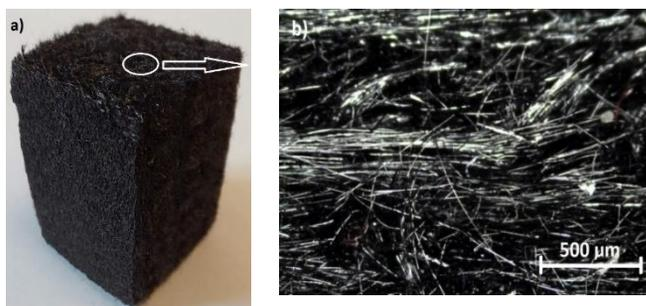
Fig. 2. View of the CF sample (a) and the microstructure (optical microscopy) of the carbon reinforcement (b)
