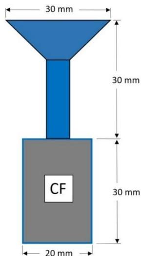
Fig. 3. Diagram of the CF insert mounted on the wax pattern of the main casting
