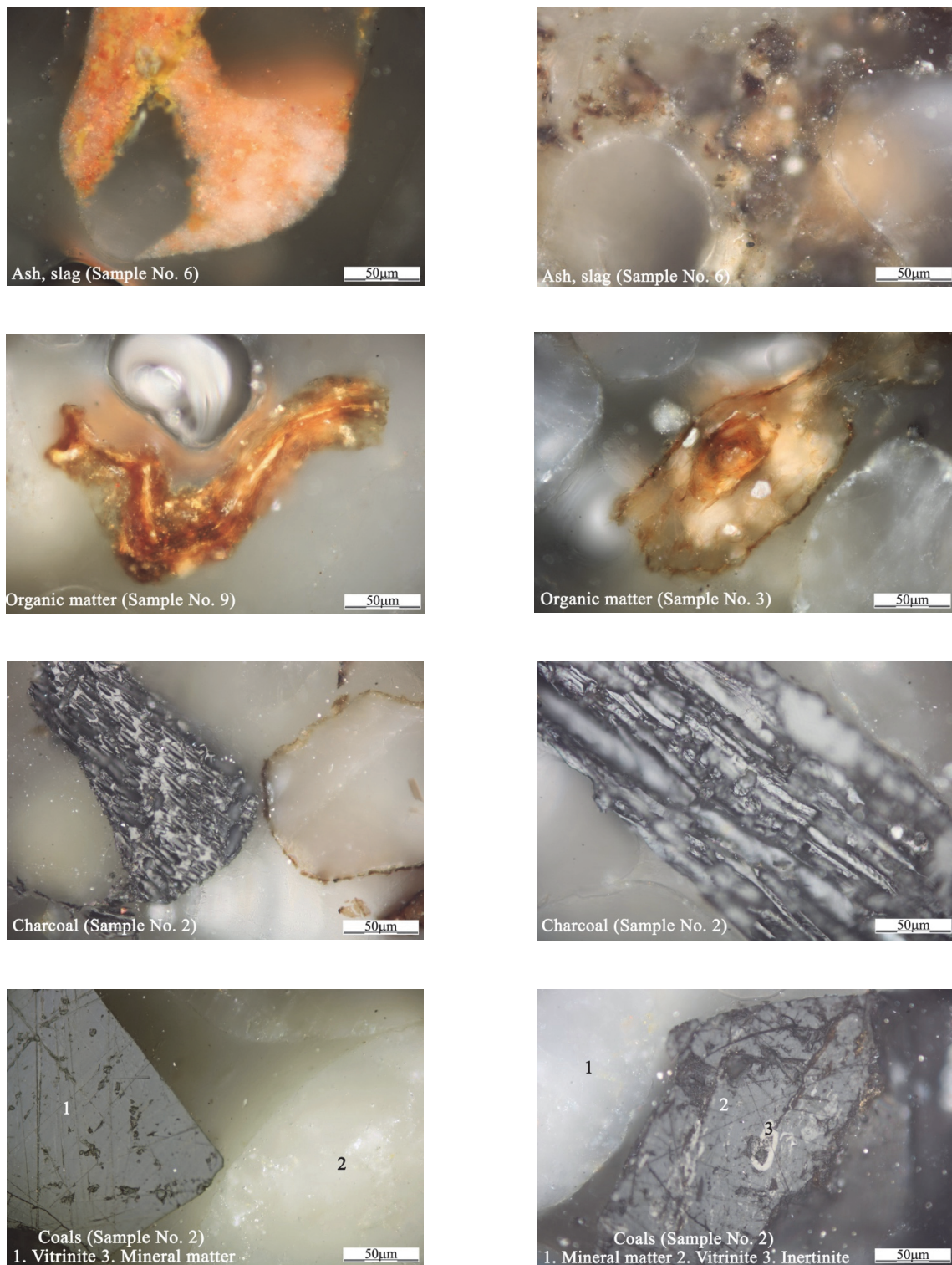
Fig. 7. Microscopic images of solid components of beach sands isolated during petrographic analysis
