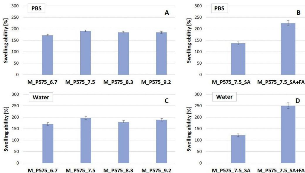
Figure 5. Swelling abilities (%) of hydrogels crosslinked with different amounts of PEGDA 575 and bio-hybrid hydrogels containing the system of thermosensitive nanocarrier-salicylic acid (T\_SA) and both salicylic acid and fluocinolone acetonide (T\_SA+FA) after tests in PBS (A, B) and distilled water (C, D).
