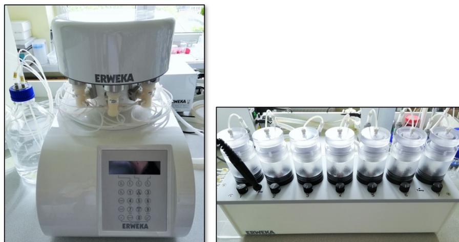
Figure 3. Photos of USP4 apparatus (DZF II Flow-Through System, Erweka GmbH, Langen, Germany).
