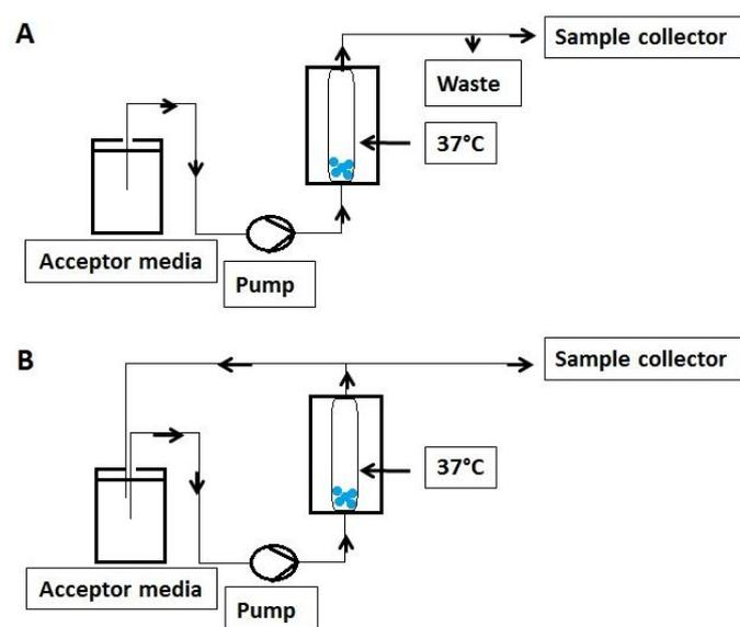
Figure 1. Schematic diagram of flow-through dissolution system: A) open mode system and B) closed mode system (adapted from Ref. (Finnie et al., 2009)).
