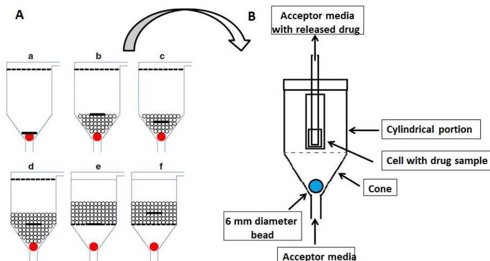
Figure 2. Schematic diagram of A – different patterns for the dissolution of films using USP4 method and B – details of a single flow chamber (adapted from Ref. (Bhattachar et al., 2002; Sievens-Figueroa et al., 2012)).
