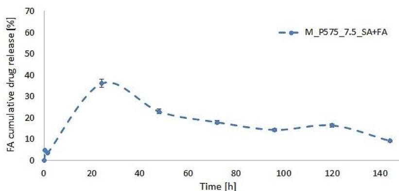
Figure 11. Release profiles of fluocinolone acetonide from the bio-hybrid hydrogel: M\_P575\_7.5\_SA+FA.
