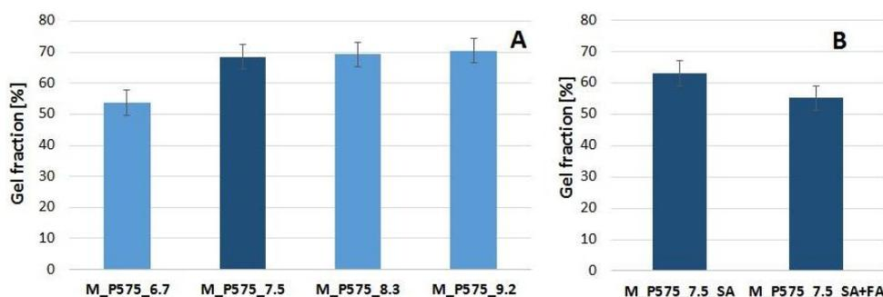
Figure 4. Gel fraction results of hydrogels crosslinked with different amounts of PEGDA 575 (A) and bio-hybrid hydrogels containing the system of thermosensitive nanocarrier-salicylic acid (T\_SA) and both salicylic acid and fluocinolone acetonide (T\_SA+FA) (B).
