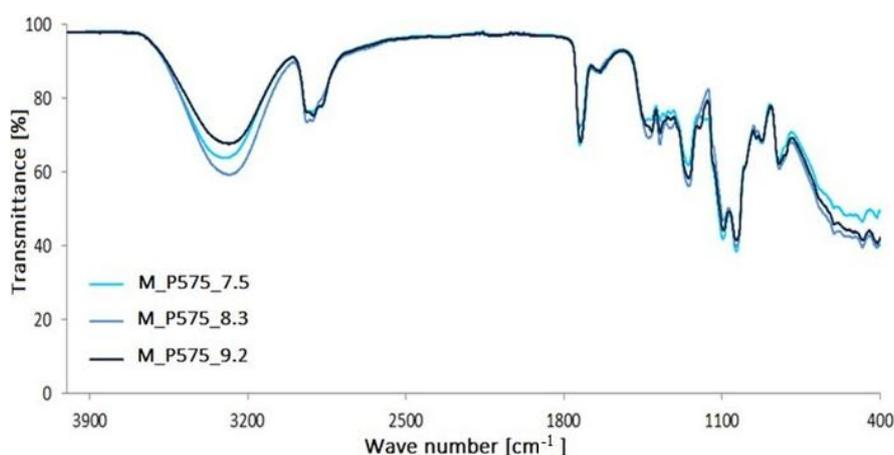
Figure 6. FT-IR spectra of hydrogels containing different amounts of PEGDA 575.
