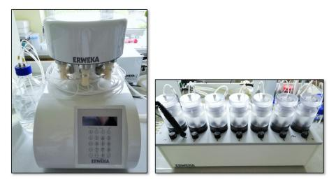
Figure 3. Photos of USP4 apparatus (DZF II Flow-Through System, Erweka GmbH, Langen, Germany).
