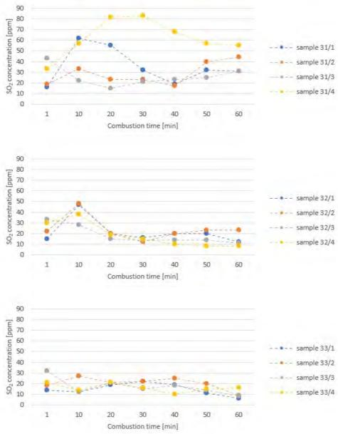
Fig. 5. SO<sub>2</sub> emission during hard-coal combustion
