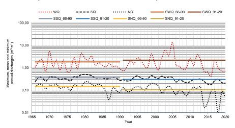
**Fig. 3.** Maximum, mean and minimum annual discharges (*WQ*, *SQ* and *NQ* respectively) at the Mławka VI river gauge in the period 1966–2020 and multiannual average of maximum (*SWQ*), mean (*SSQ*) and minimum (*SNQ*) annual discharges in the periods 1966–1990 and 1991–2020; source: own study
