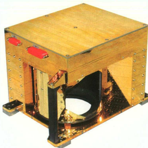
The scanner of the Polish-designed Planetary Fourier Spectrometer (PFS) aboard the Mars Express probe
