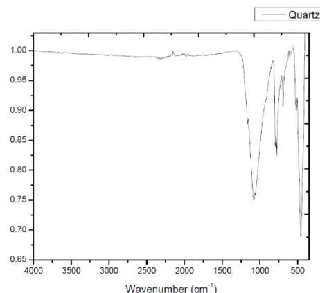
Fig. 1. FTIR spectra of Quartz
