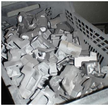
Fig. 1. Steel castings produced by investment casting
