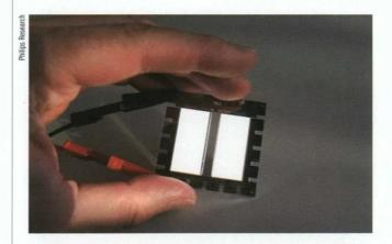
Optics are playing a major role in OLED efficiency. Only 25% of the light generated is coupled out in the forward direction if no outcoupling enhancement is used
