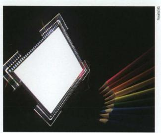
A white lab-scale OLED prototype measuring 7x7 cm<sup>2</sup>
