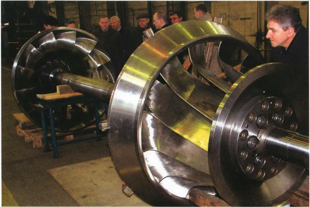
The Szwalski Institute of Fluid-Flow Machinery cooperates with water power plants – such as in coping with this defective rotor
