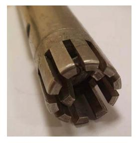
Figure 1. Homogenizer tip used to produce test emulsions.
