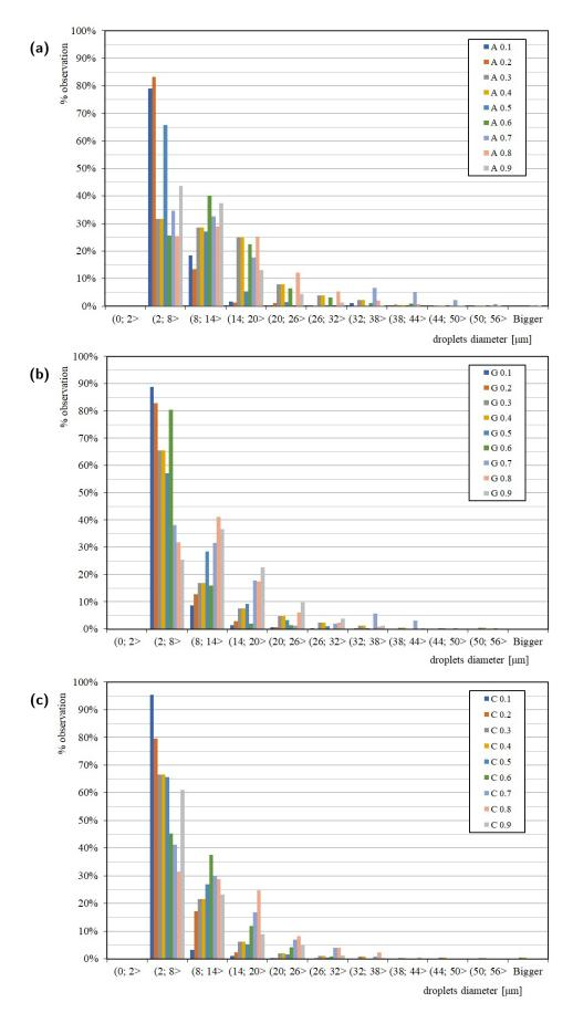
Figure 3. Droplet distributions for the tested mixtures for three glycerine to-oil ratios: a) almond, b) grape seed, c) coconut oil.
