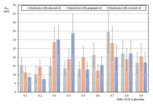
Figure 2. Dependence of average droplet diameter on the proportion of glycerine in the mixture.
