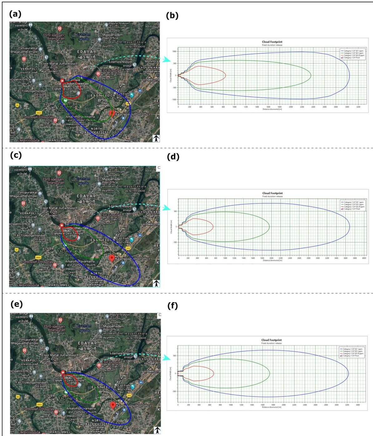
Figure 5. Threat zone area and corresponding map view at 2, 3 and 4 m/s.
