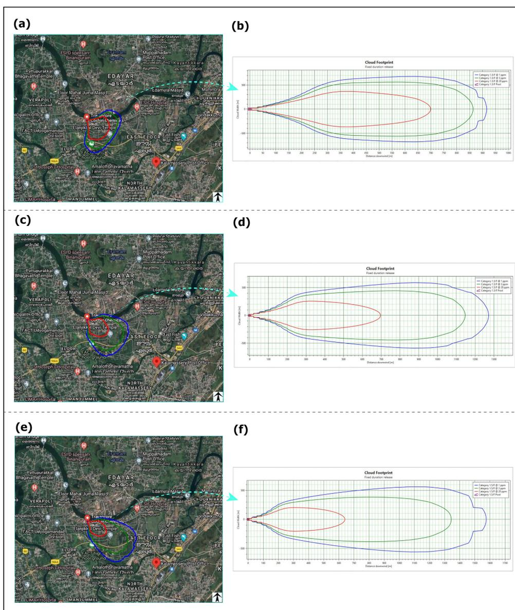
Figure 9. Threat zone area and the corresponding map view at 2, 3 & 4 m/s with the proposed mitigation system.
