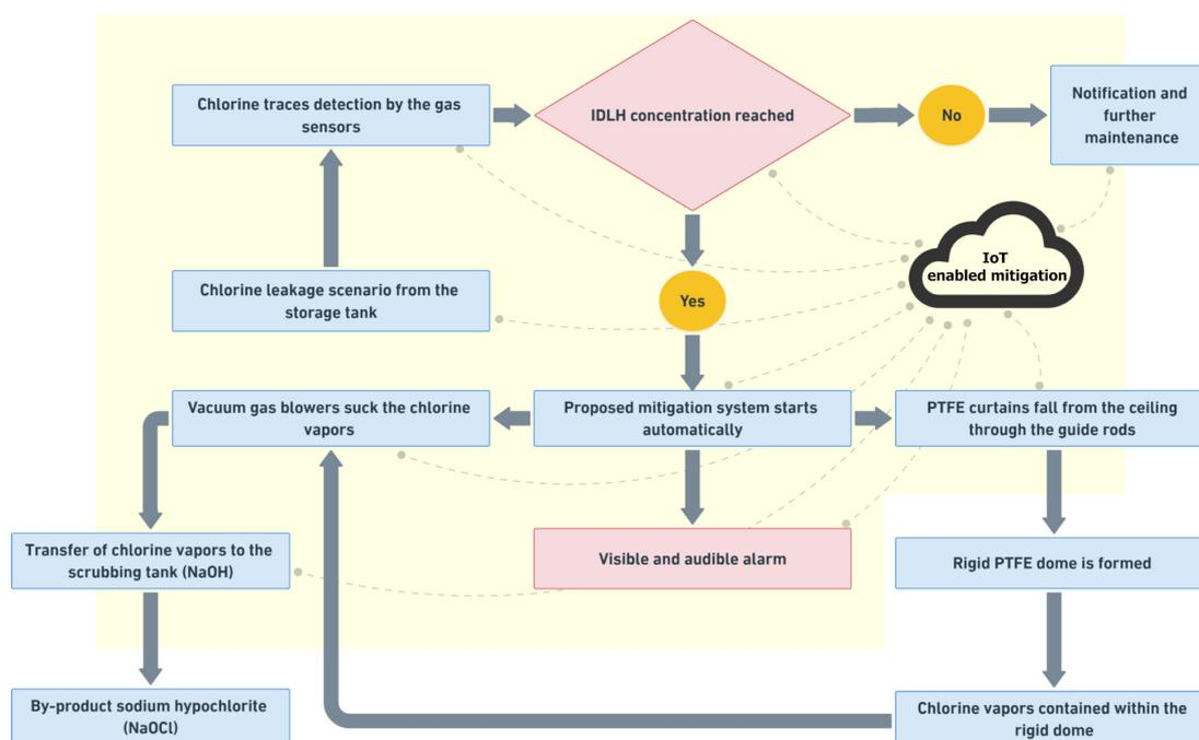
Figure 8. Flowchart of the proposed mitigation model.
