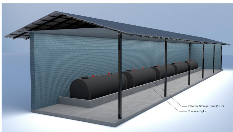
Figure 2. Schematic drawing of the storage area with dike.
