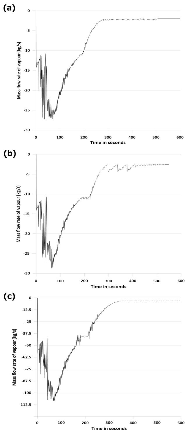
Figure 4. Evaporation rate from the pool at 2 (a), 3(b) and 4(c) m/s.
