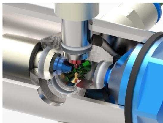
Figure 3. The detailed visualization of the liquid supply nozzles in the aerodynamic multiphase reactor.
