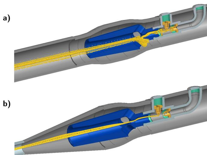
Figure 7. Comparison of the distribution of isopropanol in the stream in the case of: a) the modified design, b) the final design.
