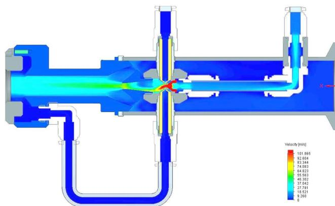
Figure 5. The designed aerodynamic multiphase reactor with an element for capturing large droplets, and also the velocity fields of the fluid flow.
