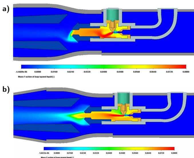
Figure 6. Comparison of the mass fraction of isopropanol in the stream for: a) the modified design, b) the final design.
