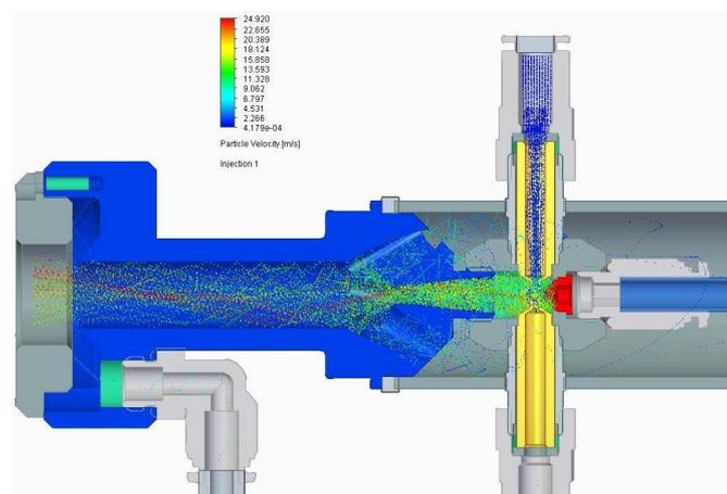
Figure 4. Movement trajectories of the droplets and their velocities for a reactor with an element for capturing large droplets.
