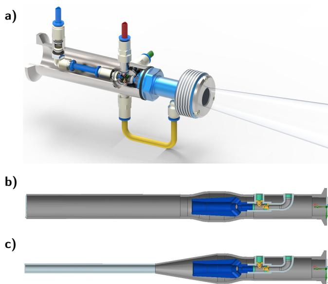
Figure 2. The designed aerodynamic multiphase reactor: a) primary construction, b) modified construction, c) final construction.
