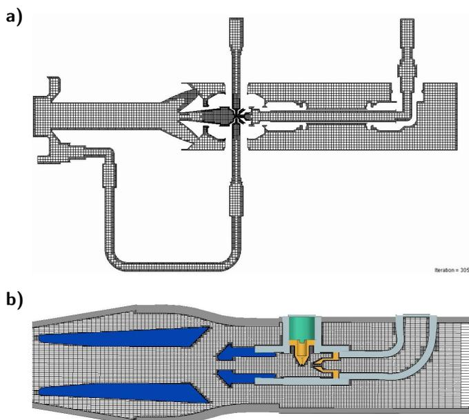
Figure 1. Mesh generated in the FLOEFD program for an aerodynamic multiphase reactor: a) with an element to capture large droplets; b) the modified structure.
