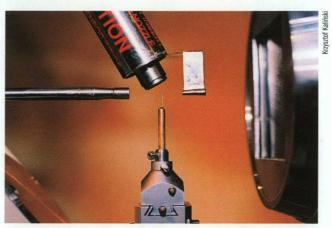
A tiny crystal on the top of the diffractometer needle is composed of several million molecules
