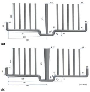
Fig. 1. Dimension of tensile mould used in the experiments (a) gravity, (b) tilt casting
