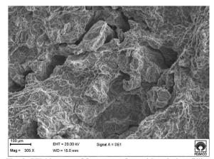
Fig. 3. SEM images of fracture surface with turbulent filling
