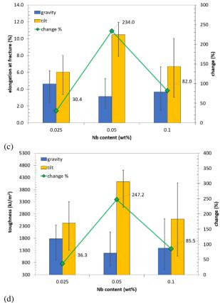
Fig. 2. Tensile property results comparing tilt casting versus gravity (a) yield stress, (b) ultimate tensile stress, (c) elongation at fracture, (d) toughness.
