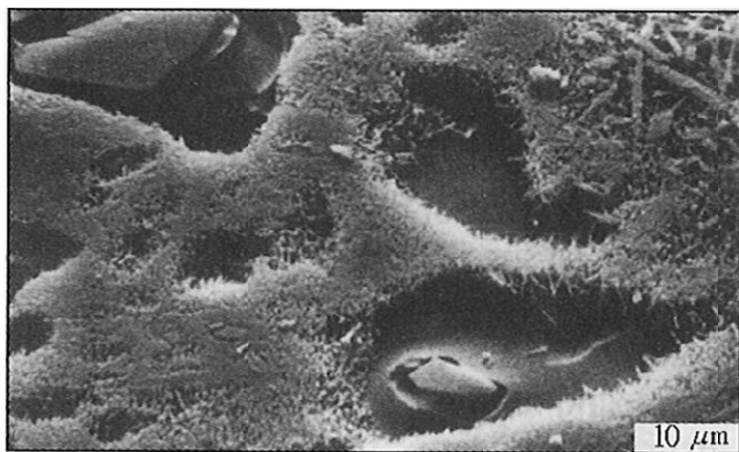
Fig. 5. SEM image of the porcelain microstructure of an unknown, probably Russian manufacturer from the turn of the 19th and 20th centuries. Melted partly and entirely quartz grains as well as matrix with numerous needle crystals of secondary mullite and small pores are visible. In the upper right corner the precipitate of secondary mullite is seen
