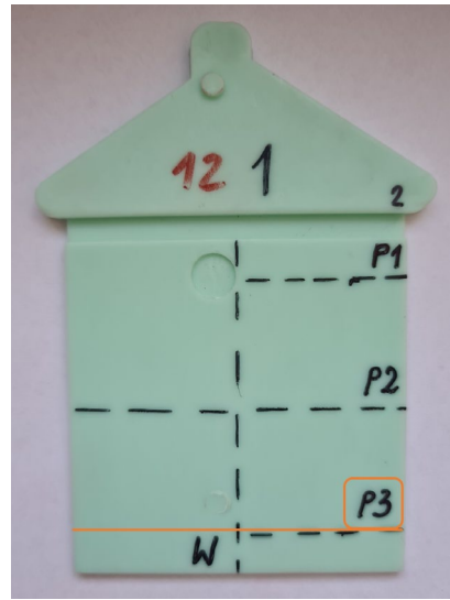
Fig. 7. Place of measuring the processing shrinkage at point P3
