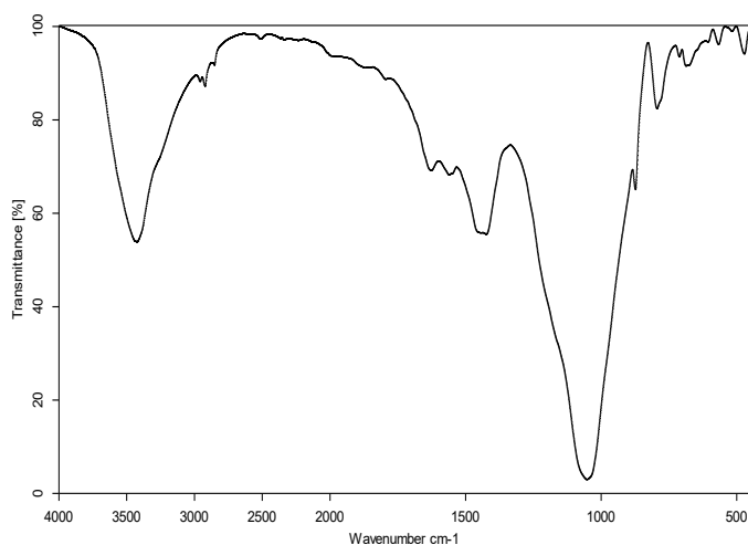
Figure 7. FTIR spectra of geopolymer PB/GEO after sorption of Zn(II) ions.
