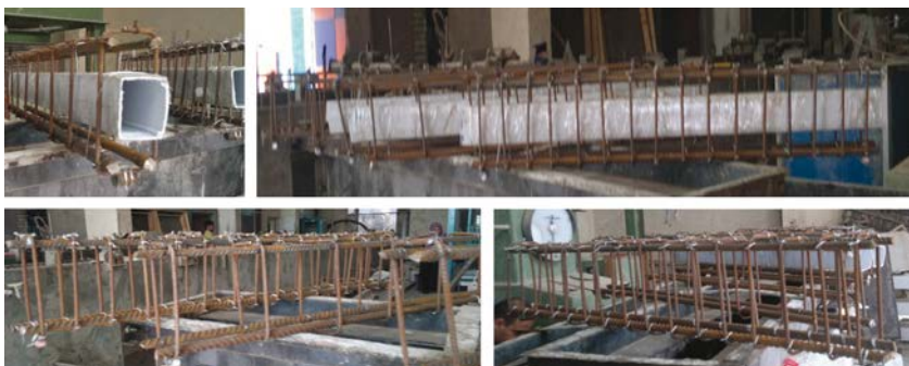
Fig. 2. Steel Reinforcement Bars and Plastic Box [4]
