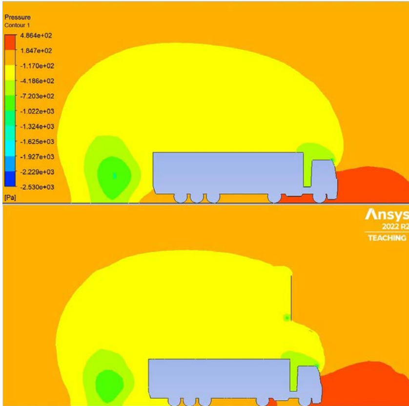
Fig. 3. Pressure distributions around a model without and with a board
