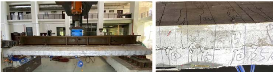
Fig. 9. Composite beam tests
